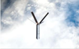
ALTAIR™ Pathfinder successfully deploying its solar arrays just after deploying from the NanoRacks CubeSat Deployer on the International Space Station. Photo Courtesy of NanoRacks and NASA.
